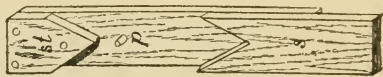
FIG. 76.—Cheshire anti-robbing entrance: st. , stationary piece; s. , slide; p. , pin or stop. (Redrawn.)
